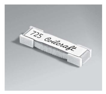
The 5315TC is Coilcraft's most rugged and lowest cost antenna coil designed for RFID applications at 125 kHz. The wrap-around terminals have large mounting surfaces to ensure excellent board adhesion. The coil is wound on a plastic base, providing great durability and allowing this part to withstand harsh mechanical shock.
